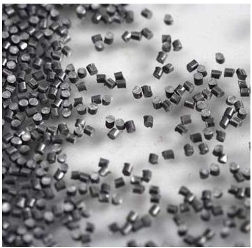
Media are propelled at high velocity during peening and blasting works. Various shot types exist for your application. Cut wire and cast steel shots can be used for both blast cleaning and shot peening while plastic media and Grit are essentially used for blast cleaning. Available in a large range of size for each type. Larger/custom sizes are available upon request.
